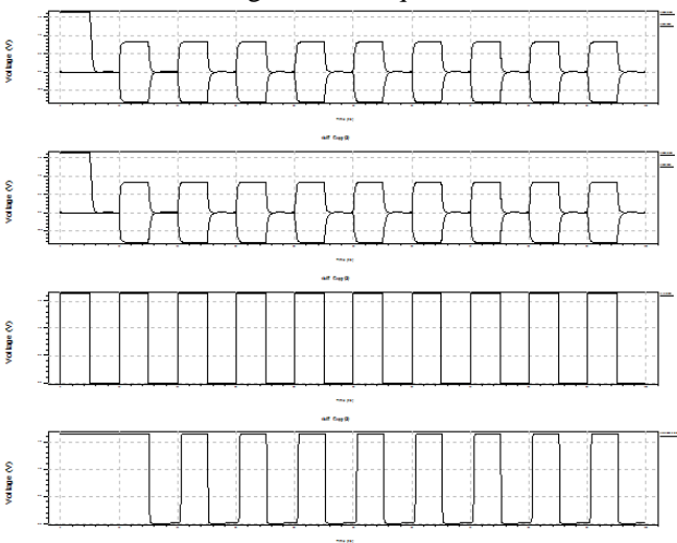
Fig .10 Simulation result for DETFF using C 2 MOS latch for half swing clock
